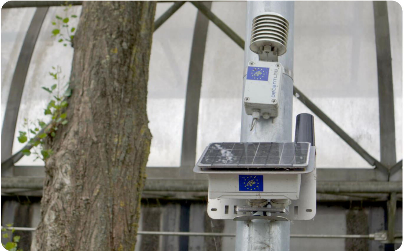
Image: A solar-powered NO2 sensor located in Wielwijk Park near the highway (May 2024) by Caitlin Ball
